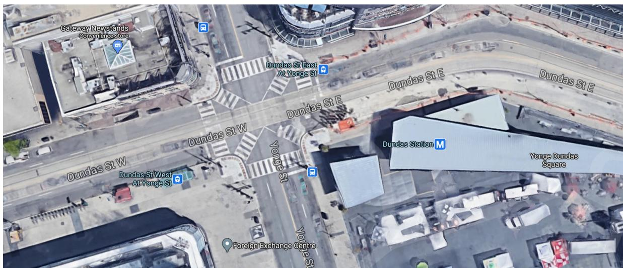
Figure 23: Aerial view of pedestrian scramble configuration, commercial land uses, and transit connections at Yonge St and Dundas St W. in Toronto (Source: [Google Maps](#))
